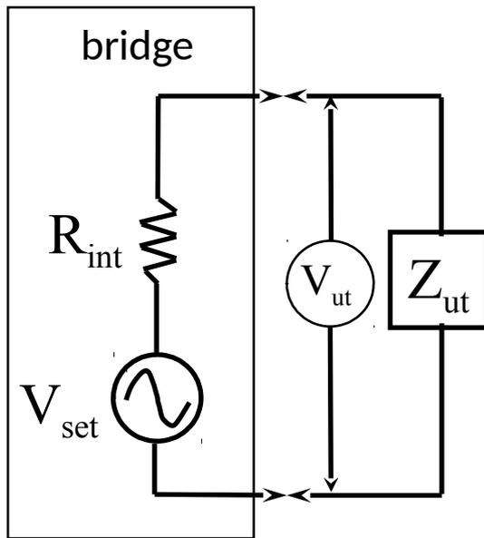
Like any oscillator or amplifier all inductance bridges have an internal driving impedance, shown here as  $R_{int}$ .
