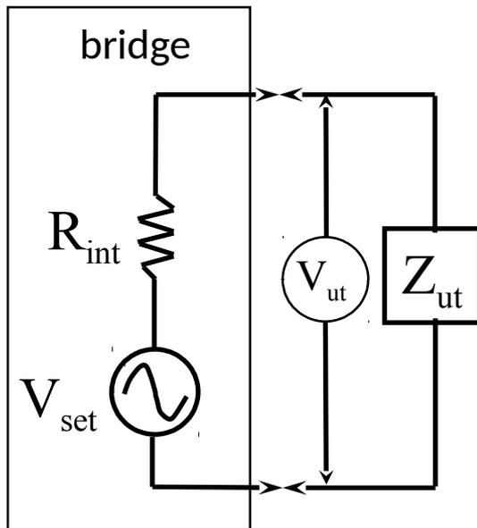
When  $Z_{ut} = R_{int}$  the voltage across  $Z_{ut}$  will be half of  $V_{set}$ .
